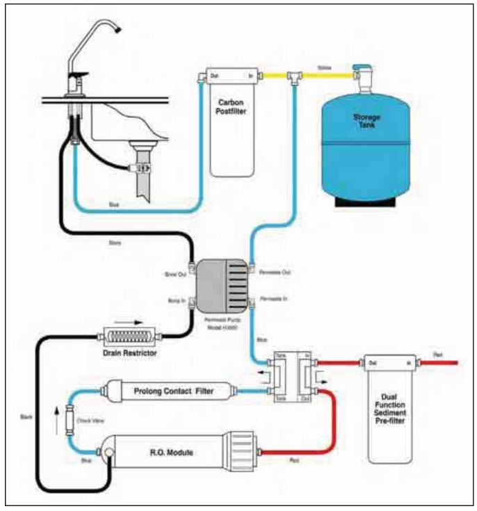
Figure 3: WaterMax® H3500 Flow Diagram
